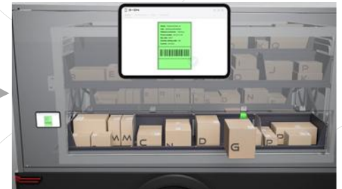
Additional package for same destination on different shelf. System knows and rotates.
