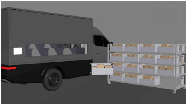
Totes are scanned into vehicle, shelf compartment
