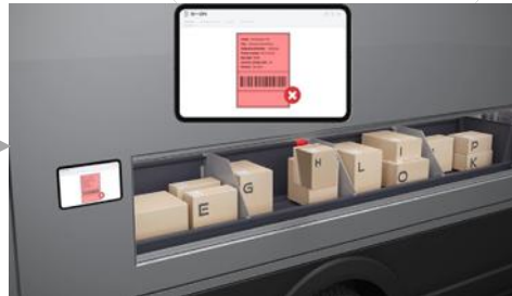
System recognizes wrongly scanned package for destination
