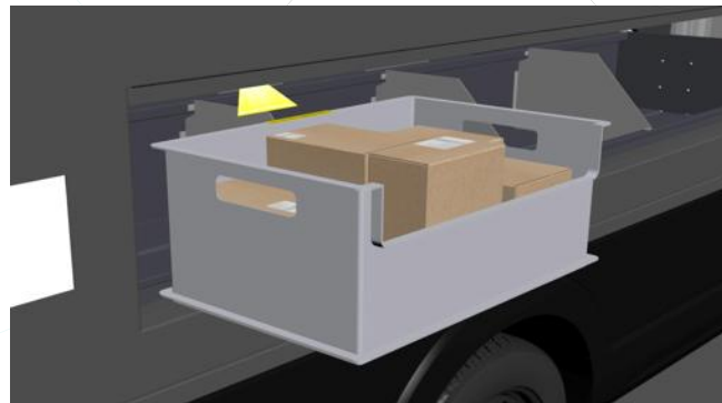
Barcode on tote initiates data information into vehicle (data is transferred form hand scanner)
